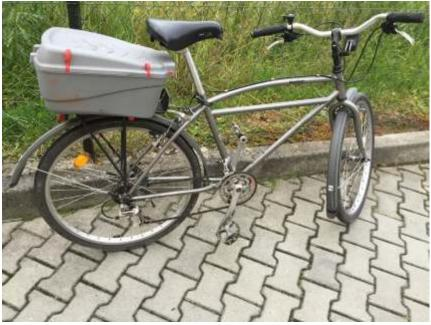
Steel wires and screws with hex nuts as well as plastic elements are all frame attachments. Assembly of the entire front and rear set takes about 10 minutes, the manufacturer provides very clear assembly instructions in four languages.
