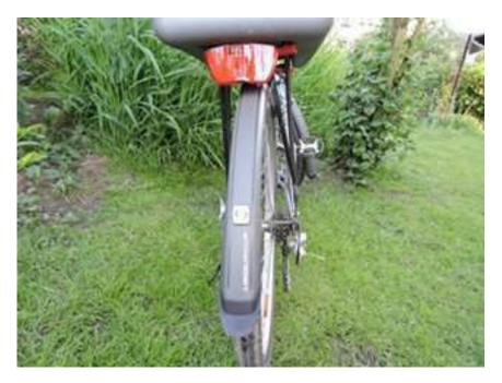
The SDL is designed to protect the entire wheel and is designed for 28-inch wheels. It is made of two types of plastic with different degree of stiffness, thanks to which the mudguard is more stable. At the end of the both, the front and rear mudguards, there is something like a rubber "splatter" - a very nice treat for the eye and added several points to the appearance of Ubiquit.
